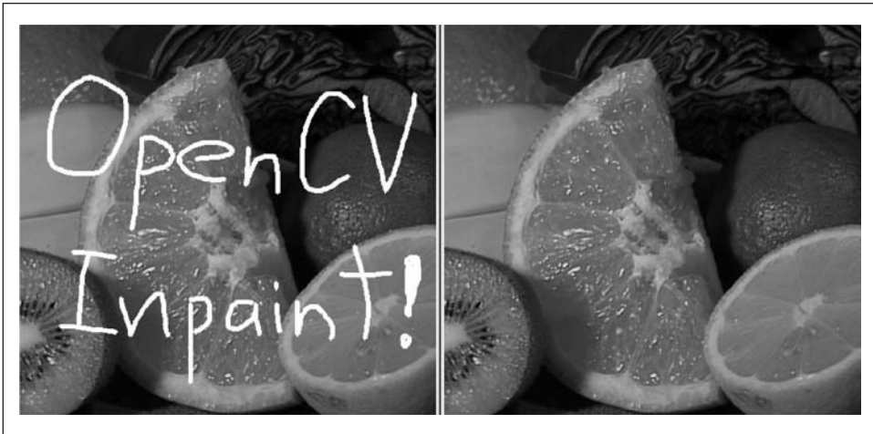
Figure 9-9. Inpainting : an image damaged by overwritten text (left panel) is restored by inpainting (right panel)
