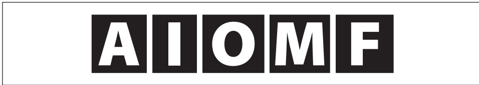
Figure 8-9. Images of five simple characters; looking at their Hu moments yields some intuition concerning their behavior
